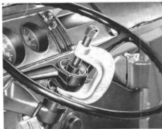
Fig. 9-14. Puller being used to remove steering wheel from pre-1975 steering column.
