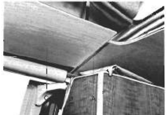
Fig. 7-19. Panel above sliding door being removed. Locating channel is at A, retaining channel at B and roof trim panel at C
