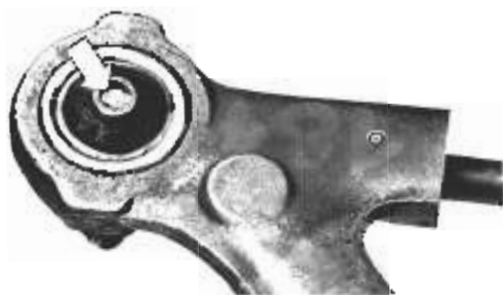
Fig. 7-2. Late-type ball joint with test surface (arrow) instead of plastic plug.
