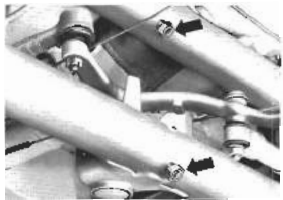
Fig. 7-15. Setscrews with locknuts (arrows) that hold the torsion bars in their center bushings
