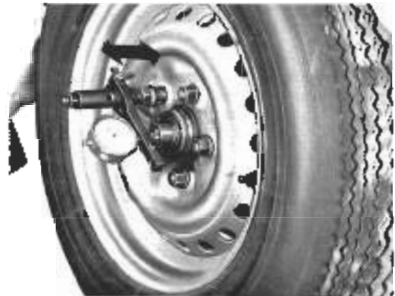
Fig. 5-2. Dial indicator being used to measure wheel bearing axial play (indicated by arrow)
