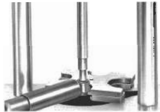
Fig. 4-1. Metal sleeve and rubber bushing being pressed out of the shock absorber.
