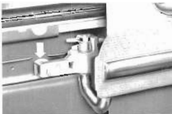
Fig. 5-35. Roller (arrow) at point with recess in the top of the center runner.
