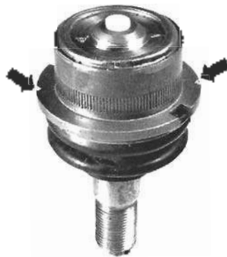
Fig. 7-9. V notches (arrows) that identify an oversize ball joint.
