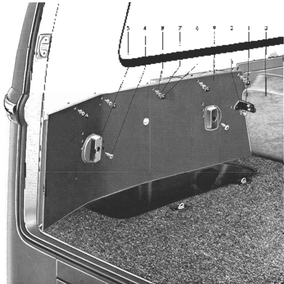
Fig. 6-7. Luggage compartment side trim panel removal.
