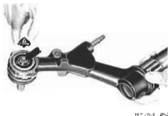
Fig. 7-3. Test point being installed. Screw the point into the hole for the plastic plug.
