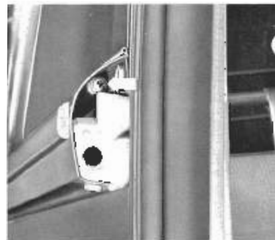
Fig. 5-34. Phillips head screw (arrow) that is inserted into the end of the retaining strip
