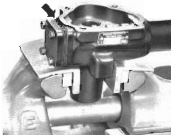
Fig. 9-21. Front (arrow) of which shims are installed.
