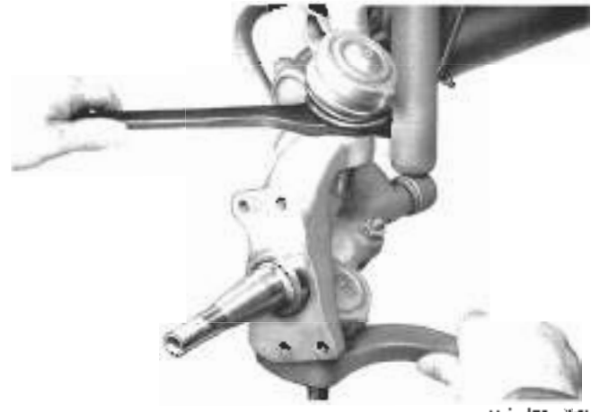
Fig. 3-3. Eccentric camber adjusting bushing turned (Wheel and brake removed for clarity).
