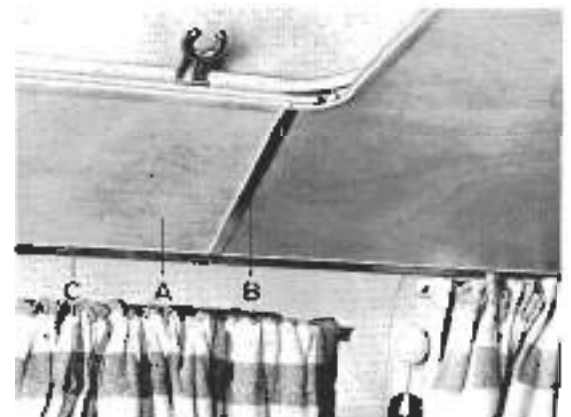
Fig. 7-20. Panel above side window and related parts. Roof trim panel is at A, locating channel at B, and retaining channel at C.
