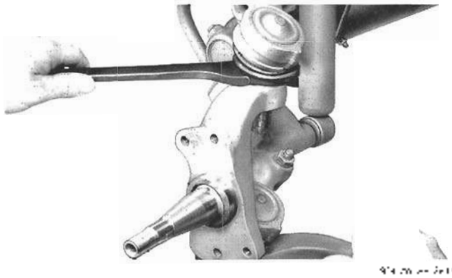
Fig. 6-4. Eccentric camber adjusting bushing being turned. Support the steering knuckle so that it does not drop off suddenly.
