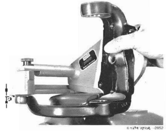
Fig. 6-9. Special gauge in position with its center plate slipped over the stub axle. Check the steering arm for a, as described in the text.
