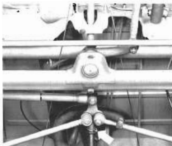
Fig. 8-1. Coupling (arrow) where gearshift rod can be disconnected.
