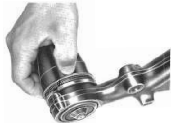
Fig. 7-7. Reaming into ball joint seal. Slide large end of conical sleeve and retaining ring. The retaining ring groove must be concentric.
