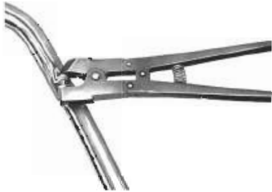
Fig. 5-28. New rivet being installed
