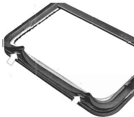
Fig. 5-60. Metal tabs that hold the vent wing frame in the sliding door.
