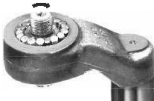
Fig. 9-19. Direction peg should be turned (arrow) when removing peg and tapered rollers.
