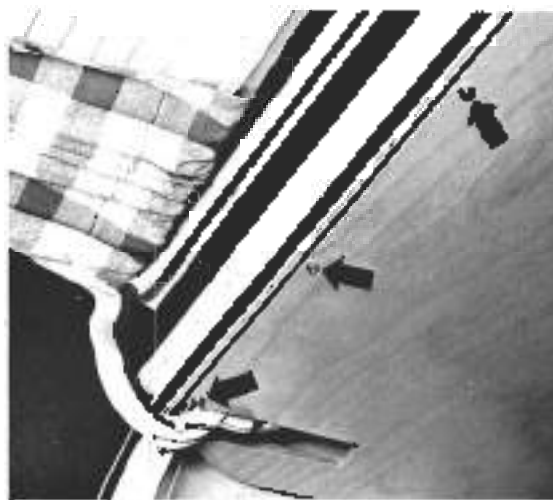
Fig. 7-18. Three of the five screws (arrows) that hold shelf to the roof frame. Luggage compartment lid must be raised for access to the screws
