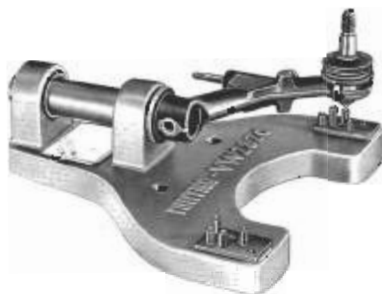
Fig. 7-4. Early-type ball joint. Test point should contact the boss on test plate.
