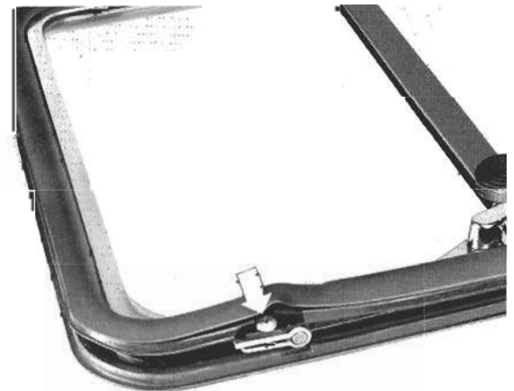
Fig. 5-61. Metal tab(s) that must be removed before you can take the vent wing out of its frame.
