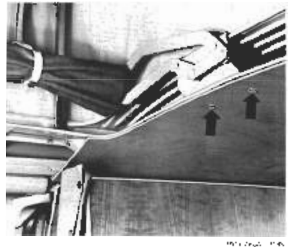
Fig. 7-24. Folding cot screws with self-locking nuts (arrows).
