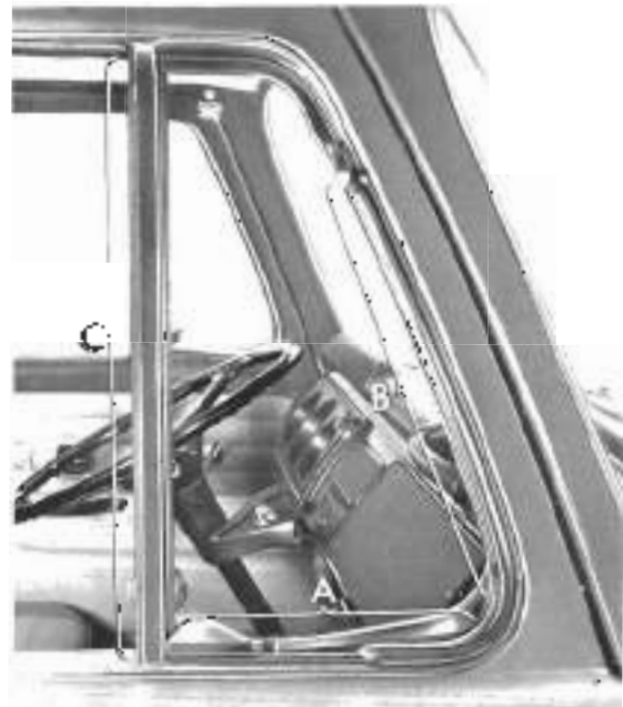
Fig. 5-30. Points for checking vent wing alignment
