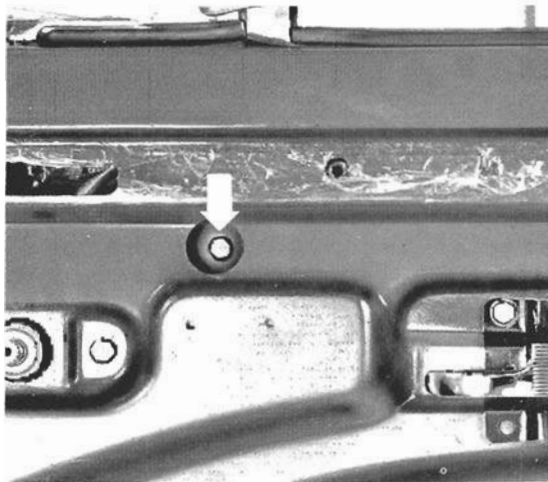
Fig. 5-24. Cap nut (arrow) for access to guide channel ball
