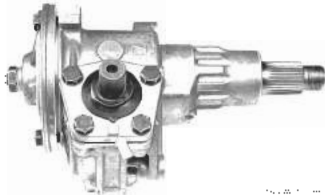
Fig. 9-5 Square boss (arrow) that pointer on dust cap must be toward when the steering is centered
