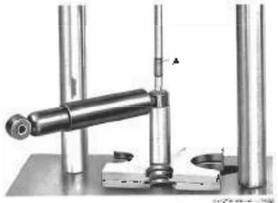
Fig. 4-2. Metal sleeve being pressed in.
