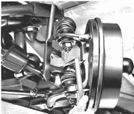
Fig. 7-1. Lever and vernier caliper in position. Lever should draw the two torsion arms toward one another when the handle is raised.
