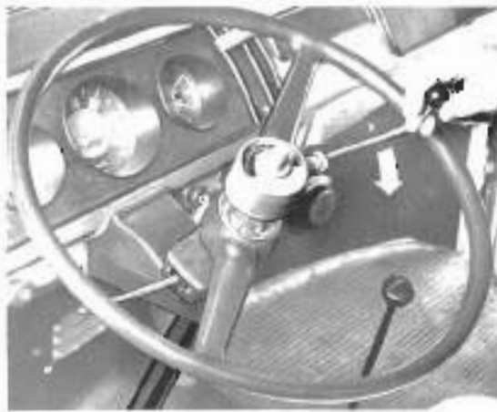
Fig. 9-4 Torque gauge being used to check wheel and pin steering adjustment
