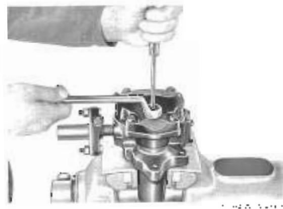
Fig. 9-25. Locknut being tightened while adjusting screw is held stationary with screwdriver.
