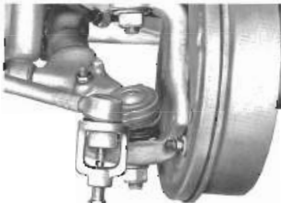
Fig. 9-6. Tool used to press out tie rod ends
