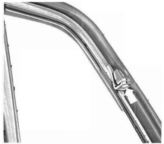
Fig. 5-27. Rivet that holds the vent wing to the vent wing frame. Grind the end of the rivet at the point indicated by the arrow
