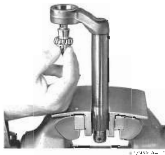
Fig. 9-22. Peg with tapered rollers being installed in peg shaft.
