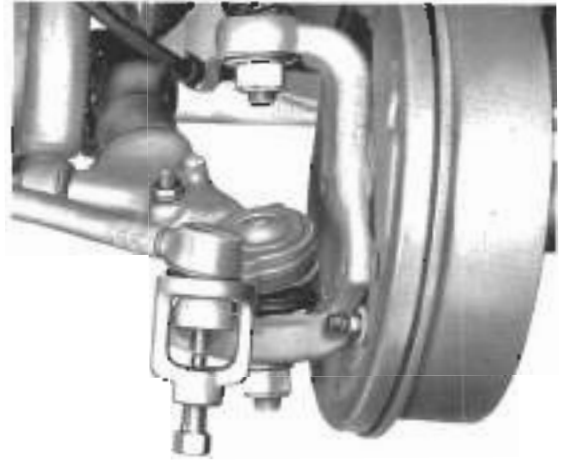
Fig. 6-2. Tie rod end being pressed out. The tool shown prevents damage to the threads on the tie rod end stud.
