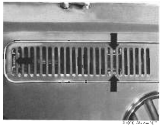
Fig. 10-4. Phillips head screws (arrows) that hold air intake grille and mesh panel
