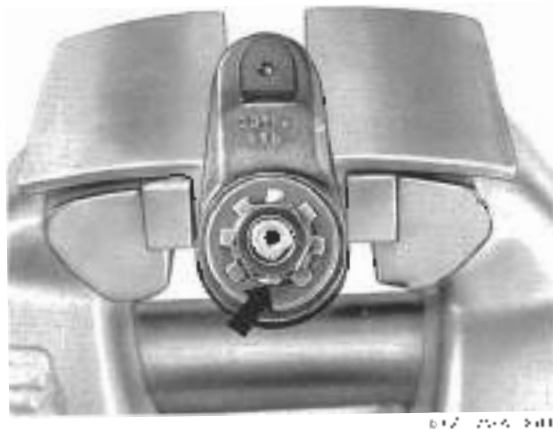
Fig. 9-23. Tab on star washer (arrow) bent over against the top of the nut.
