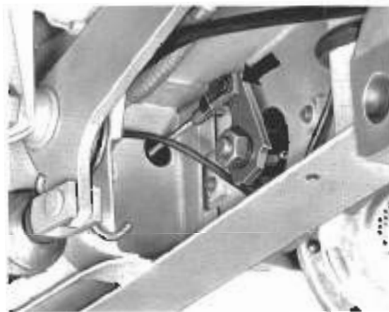
Fig. 8-2. Clutch cable disconnecting point (arrow).
