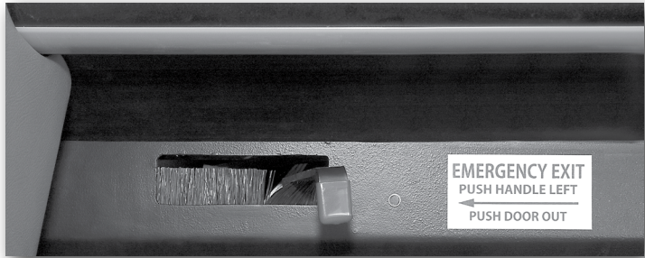
Electric Door Release Lever- Closed Position
