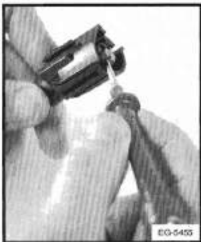
Figure 6-20. - Remove Lock Wedge
