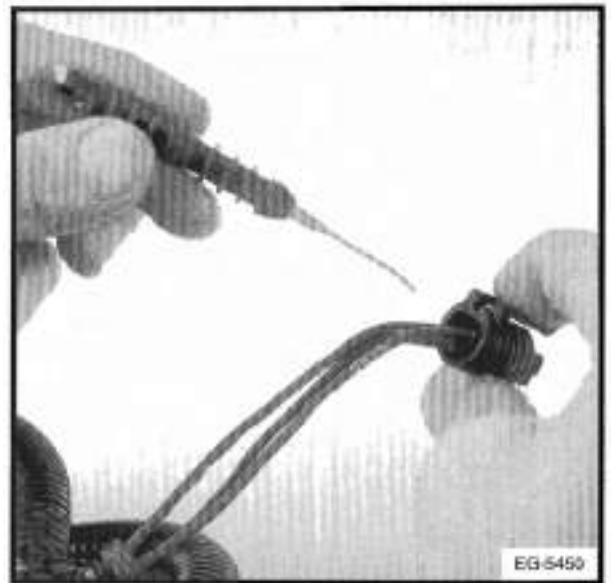
Figure 6-31. - Release Terminal Lock Tab
