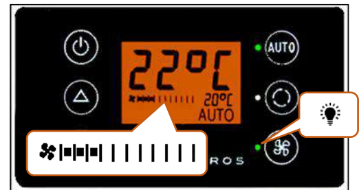
Figure 10 - SC600 setting the blower level manually
