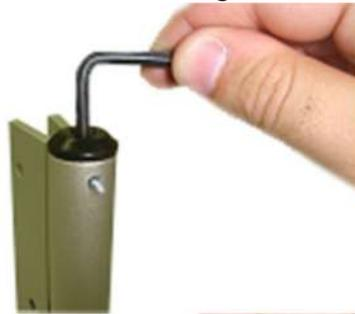
Remove the pin and tight bolt to left in  $\frac{1}{4}$  of turn.
