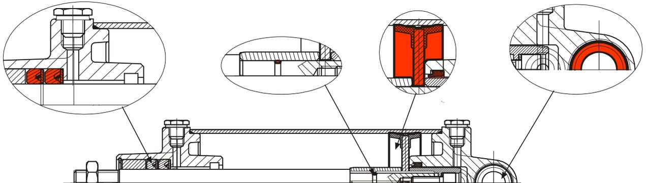
Replace the cylinder consumable parts by using a cylinder repairing kit if necessary.
