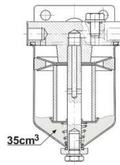
**2.6.2 HOWEVER, A BLEND OF SAE 10 PLUS 5% OF BISULPHIDE CAN ALSO BE APPLIED**
