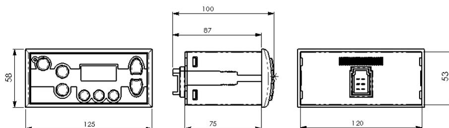
For the installation of the CPU, the arrangement of the fixing holes must be taken into account, as shown in the figure.
