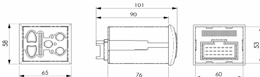
On the rear of the unit there is an AMP Timer Power Junior connector with 21 pins, ref. AMP 966140-6. The connector to be used in the electrical installation is that with ref. AMP-1-0967625-1. The receptacle terminals have ref. AMP 927775-3.
