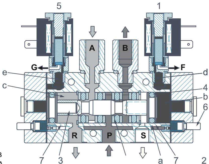
The 5-way 2-position electrovalve conveys the pneumatic air flow to the corresponding opening or closing chambers of the actuating cylinder, while connecting the inactivated cylinder chamber with the atmosphere.
