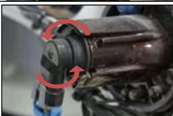
Remove the head light lamp by turning the lamp support
