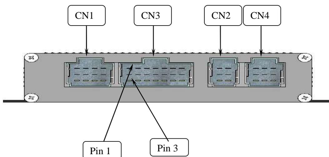
The references of the electric installation connectors for the CPU are as follows:
