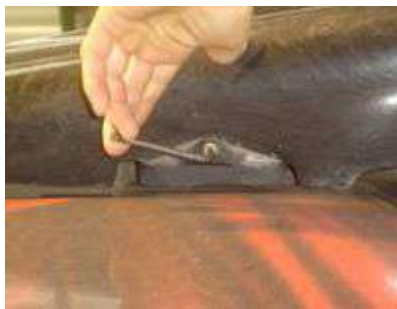
Remove the fixing screw – Allen 5
