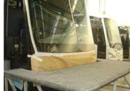
Masking paper on front dome
