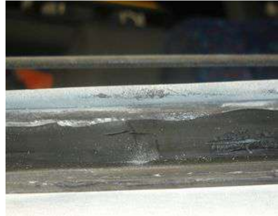
Remaining Adhesive layer (1 to 2mm thick)
