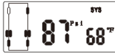
▲ Left front wheel ID successfully written into the hose
