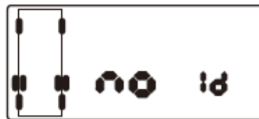
▲ No-code module alarm occurs at the left front wheel position
