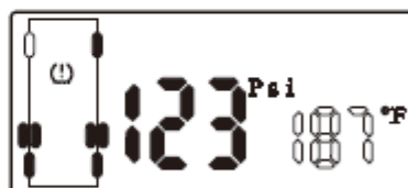
▲ High-temperature alarm occurs at left front wheel position
